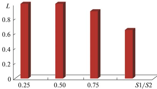
**Fig. 4.** The noise level diagram generated during interaction of rings with various ratios of working areas.  $S1/S2$  is the ratio of the working areas of the rings and  $L$  is the relative noise level (1.0 corresponds to the highest total noise level for  $S1/S2 = 0.25$ ).
