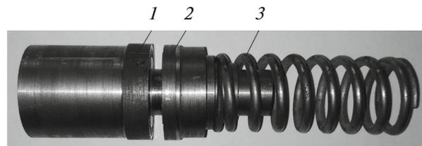
**Fig. 3.** Loading device: (1) stationary ring, (2) mobile ring, and (3) spring with specified stiffness.
