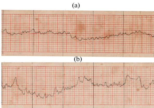
**Fig. 2.** Intrinsic surface profilograms recorded in the application area of compression stresses (+): (a) is the surface profilogram of a brake disc before loading and (b) the surface profilogram of a brake disc during loading with normal and tangential forces.
