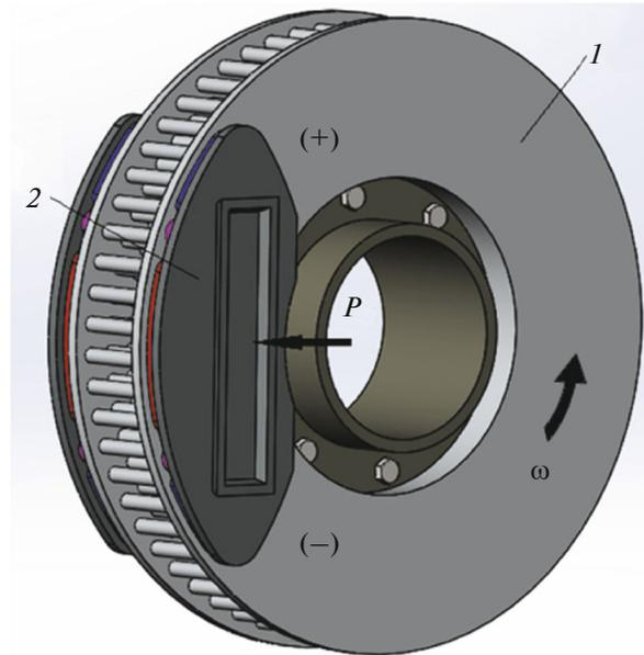
**Fig. 1.** The loading diagram of a disc brake during application of the brake: ( $I$ ) brake disc; ( $2$ ) brake pad;  $\omega$  is the rotation rate of the brake disc; (+) is the region of deformation of the microgeometry; (–) is the region of elastic recovery of the microgeometry; and  $P$  is the pressing force of the brake pad to the brake disc.
